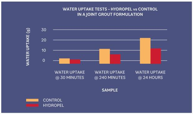
\*The use of Hydropel results in achieving a grout class of CG2W according to BSEN 13888 - Table 7.
