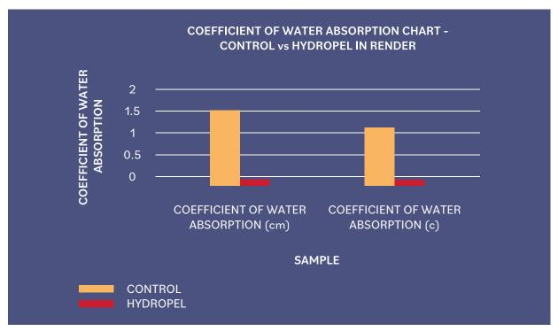
The use of Hydropel results in achieving a grout class of W2 according BSEN 998 -1 Table - 1.
